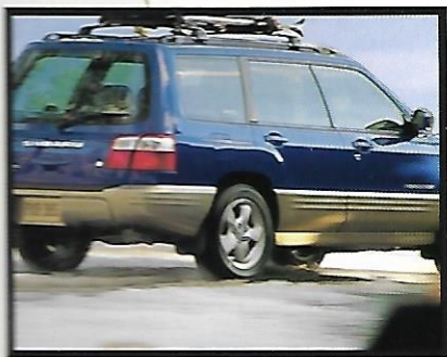
When accelerating, the vehicle's weight shifts rearward, reducing the traction of the front wheels. In response, Subaru AWD directs power to the rear wheels where there is more traction.
