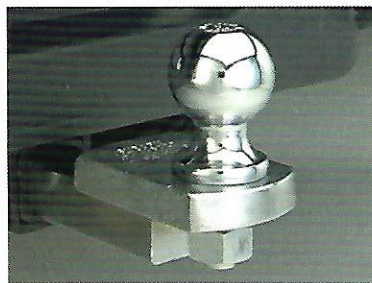
Trailer hitch. Heavy-duty-rated at 200 lbs. tongue weight, 2,000 lbs. towing capacity (ball not included).
