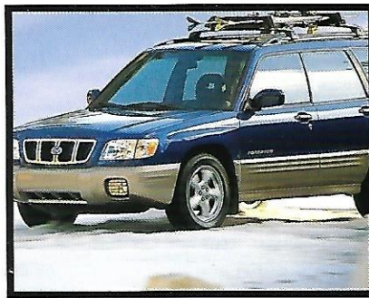
When braking, the vehicle's weight shifts toward the front, reducing rear-wheel traction. Subaru AWD responds by sending power to the front wheels for better steering control and braking performance.
