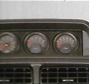
Manifold vacuum gauge pack. Displays manifold vacuum, voltage and temperature.
