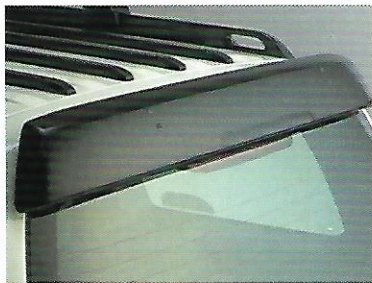
Rear window dust deflector. Helps keep back window clear of dust and debris.
