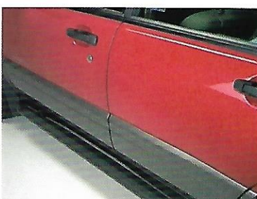
Side underguard bar. Helps protect side of vehicle, while providing a nonslip step to help reach roof of vehicle. Not applicable for vehicles with side air bags.
